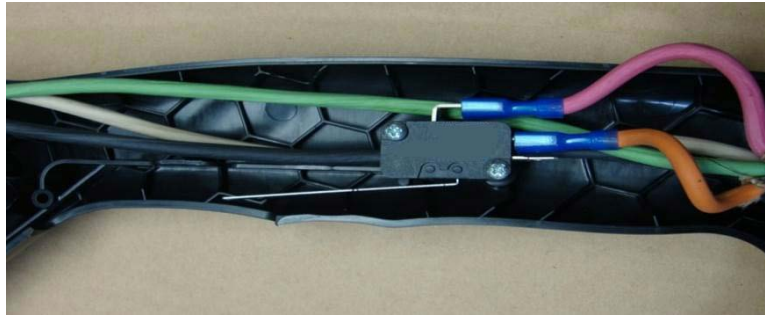
Fig. 6-15 Switch Wire Location
